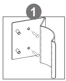
Attach right side of bracket to cart first, using included screws.
