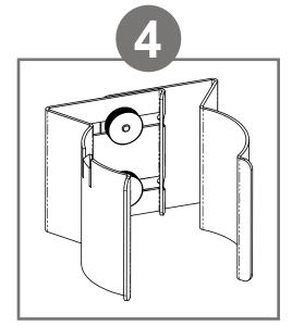
Determine size needed for disposable wipe canister and tighten plastic knobs at position needed to accommodate canister.
