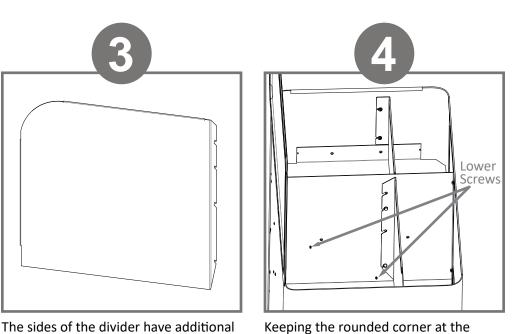
Keeping the rounded corner at the top left, reposition divider at a slanted position, resting on lower screws.
