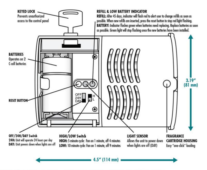
Operates using 2 C cell batteries; Alkaline recommended; batteries last up to 16 months.
