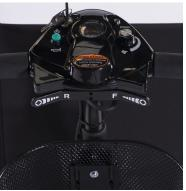
The modular control panel works seamlessly to provide precision speed adjustment and an intelligent, safe braking system.
