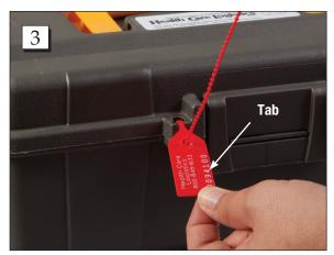
**Step 3.** Utilize the "TUG" test by grasping the tab of the seal, gently tug on it to determine closure. If you are able to loosen the seal, IT IS NOT FULLY LOCKED. Remove the seal and replace with a new one.
