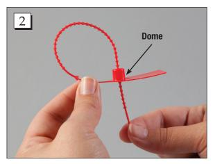
**Step 2.** Pull the stem through the locking dome on the sided marked "Enter". Pull it as tight as possible around the item being sealed. This will ensure that the seal stem cannot be broken and reinserted into the locking mechanism.
