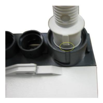
22. The plug must be pushed in flush with the controller. If there is any difficulty when inserting the plug a very small amount of petroleum jelly on the rubber O ring is required or remove the O ring.
