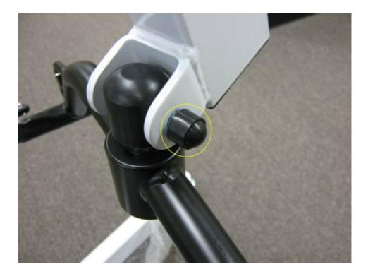
21. Align the tab on the plug of the hand control with the indent in the hand control socket.
