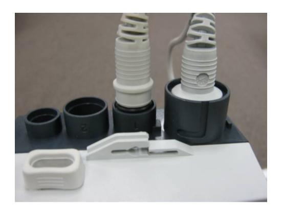
24. The plug must be pushed in flush with the controller. If there is any difficulty when inserting the plug a very small amount of petroleum jelly on the rubber O ring is required or remove the O ring.
