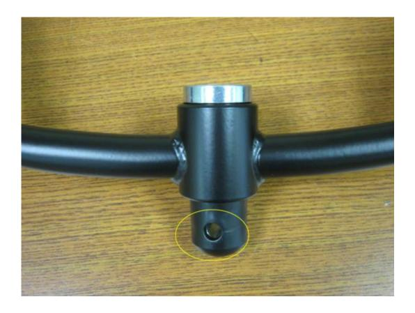
18. Align the holes of the cradle pin and cap with the holes in the U bracket at the end of the boom. Insert the bolt through the holes.
