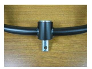
17. Install the nylon cover over the cradle swivel pin and line up the holes of both.
