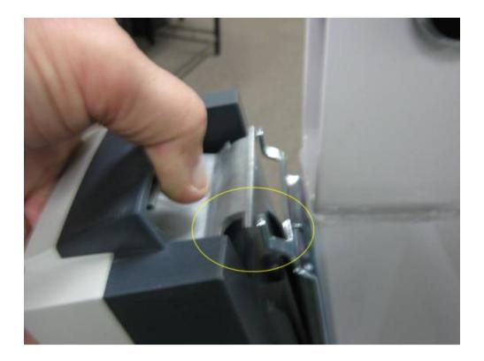
13. Push the battery pack over the upper bracket and release the locking latch to lock in place.
