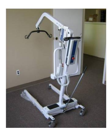
26. Charge the unit by plug the charger cord into the controller and a wall socket. The amount of charge on the battery is indicated by the bar gauge on the front of the unit. The charger plug must be disconnected from the lift for the lift to work.
