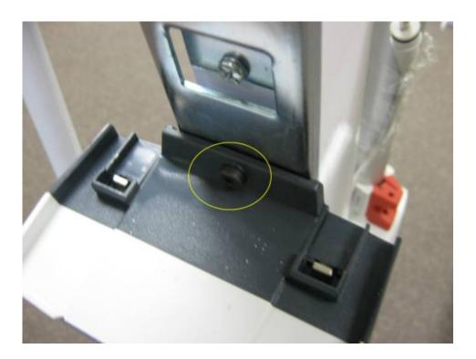
11. Line up the battery pack with the control box.
